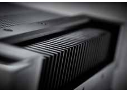
△ AMPLE HEATSINKING RUNS MILDLY WARM, INDICATING HIGH BIAS OPERATION IN LINE WITH GRYPHON'S AMP IDEOLOGY.
