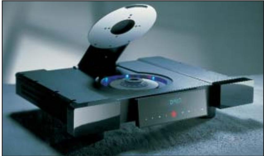
Gryphon Audio Designs take an uncompromising approach to these serious issues in the Gryphon Mikado. Instead of letting the oscillator at the CD transport generate the overall master clock, which would result in mechanical and electrical jitter, we place an ultra-low jitter oscillator at the DAC, while a second separate local master clock controls the transport.
