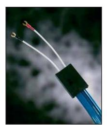
Gryphon PSC Reference (Planar Speaker Cable) consists of two solid planar conductors of gold-embedded silver equivalent to normal wire with a cross section of 4 square millimeters. Planar configuration with significantly increased surface area provides crucial electrical advantages. Each flat, wide conductor is insulated by a rigid outer jacket which also reduces sensitivity to external vibration and for optimum signal transfer, Gryphon PSC Reference includes a custom termination box.
