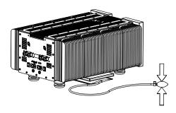
Remove sliding-sheet and shock absorbing feets.
