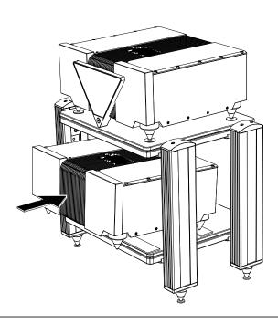
4. Put down the front end spikes at the felt.
