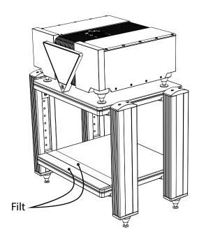
2. Put down the rear end on the most rear piece of felt.
