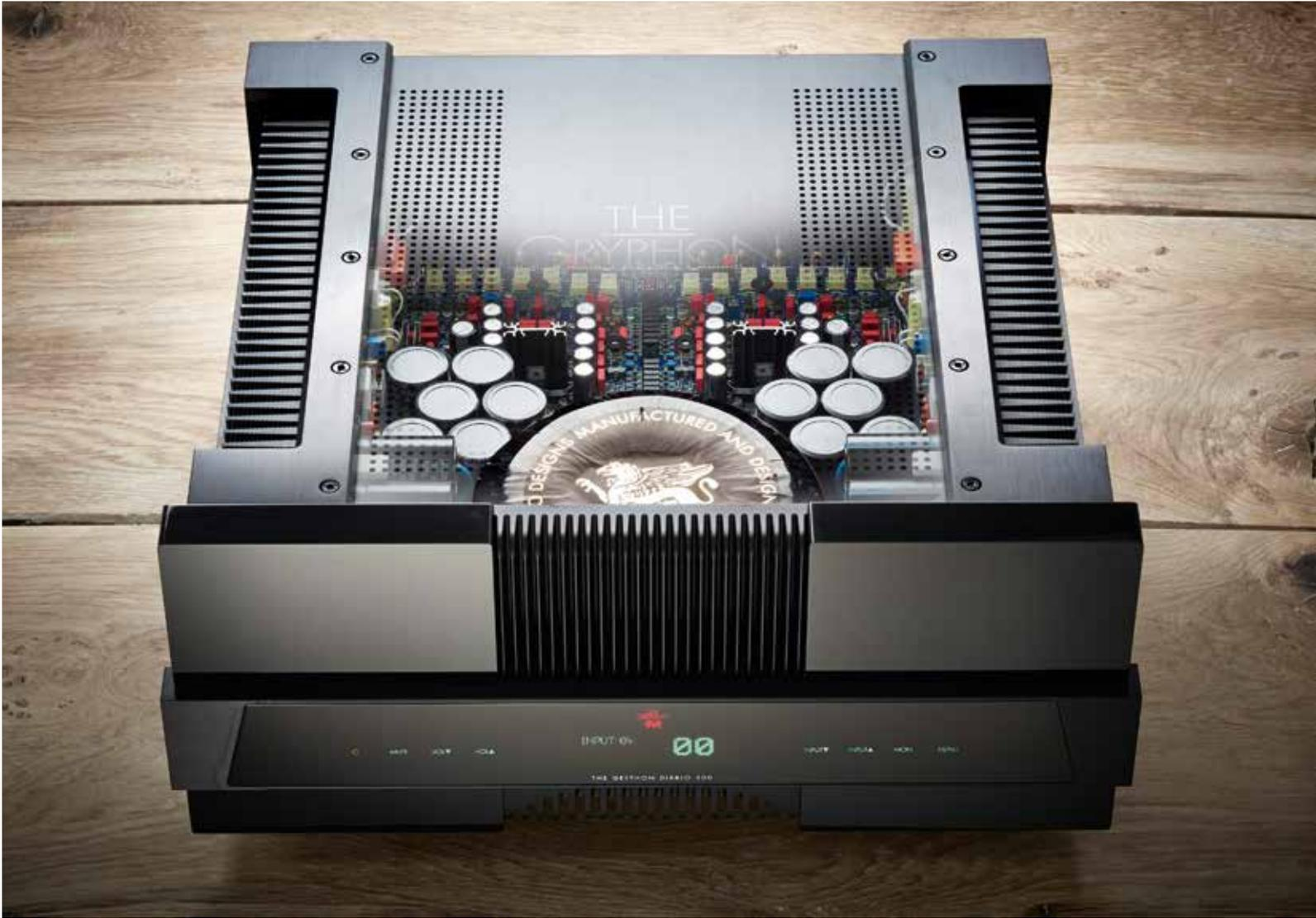
△ WELL-ENGINEERED POWER SUPPLY FEATURES A LARGE CUSTOM TRANSFORMER AND MULTIPLE CAPACITORS STORAGE.
